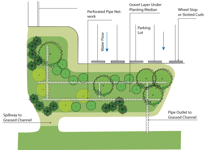
Raingarden example with underdrain
